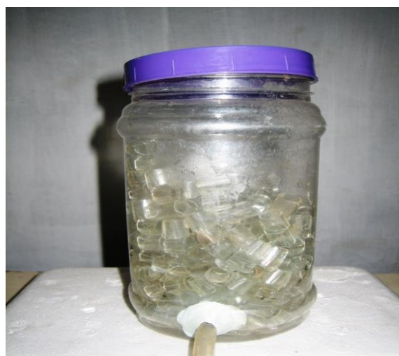
Photograph 2: Indigenously prepared fixed film bioreactor
